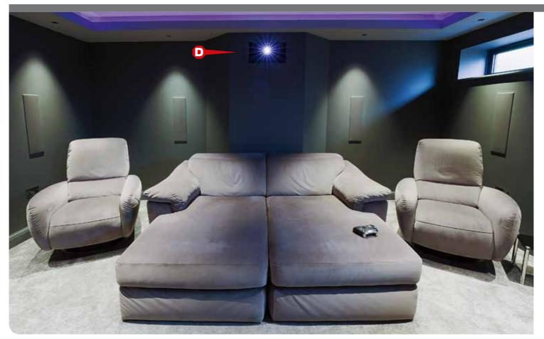
**D. Firing further** A mirror system is used to create a 3m-wide image from the cinema's Epson projector – which is mounted vertically within this false 'chimney'
